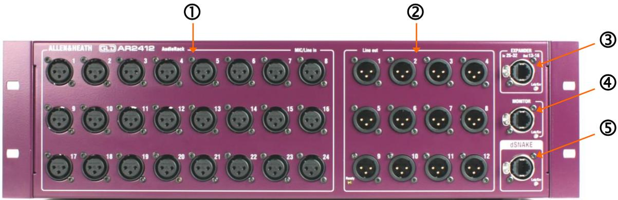
**① Input sockets** 24 balanced XLR inputs for microphone and line level sources. The preamps are built into the AR2412 rack and their Gain, Pad and 48V phantom power is remote controlled from the mixer via the dSNAKE link. The output of the analogue preamps are converted to digital format and transported via dSNAKE to be processed and mixed at the GLD or Qu mixer.
