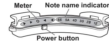
2. Play a single note on your instrument. The note name indicator will light up that's closest to the pitch detected. Tune your instrument to the correct pitch so that the desired note name lights up.
