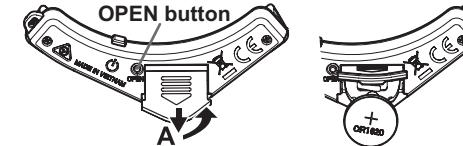
2. Making sure to observe the correct polarity, insert the battery so that the "+" side of the battery is visible.
