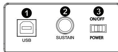
**NOTE:** The polarity of the sustain pedal is determined by the keyboard upon startup. When Keystation is powering up, the sustain pedal is assumed to be in the "up" (Off) position. It is important that the sustain pedal is not pressed during startup, otherwise the pedal will reverse its operation, and notes will sustain when the pedal is not pressed.
