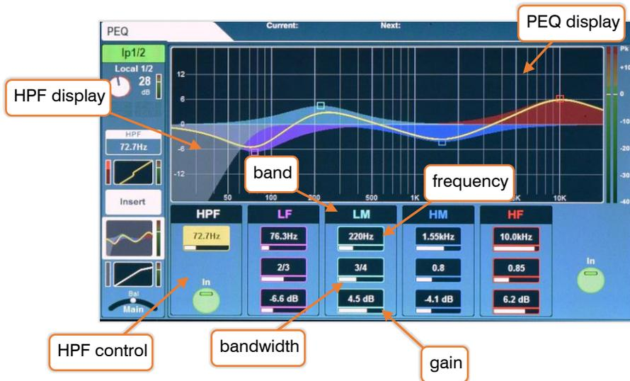
**HPF** - In order of processing, the High Pass Filter (HPF) is located post-preamp (as in the channel overview). It is displayed in the EQ screen for convenience.
