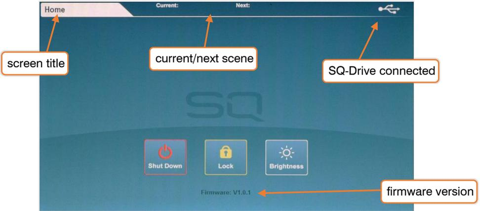
This is the first screen shown when powering on the SQ. It is also shown when no channels are selected, and no other screens are active. The firmware version is displayed below three buttons.
