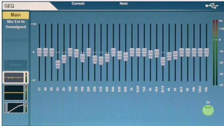
All mix channels feature a 28-band stereo graphic EQ. With a mix channel selected, and GEQ active, the green 'In' LED in the GEQ section (below the PEQ rotaries) will illuminate.
