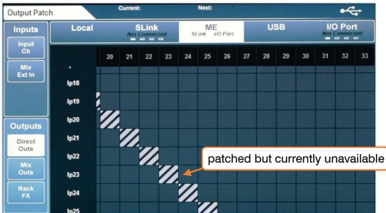
The ME patching is applied to either the SLink port, the I/O Port, or both.
