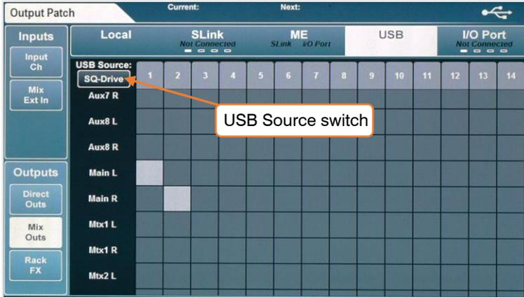
The 'USB Source' switch displayed at the top left of the matrix shows the current mode.
