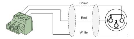
For balanced line output connections:
