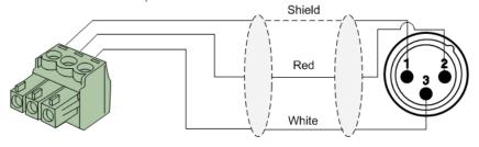
For unbalanced line in & output connections:
