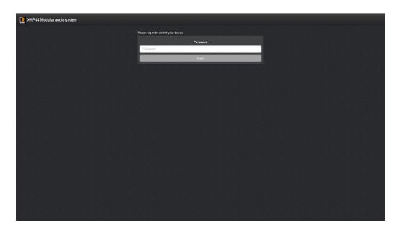
When accessing the web—control interface of the XMP44, a password should get entered to control the functions of the system. Two different levels are possible for **administrator** and **user** access.
